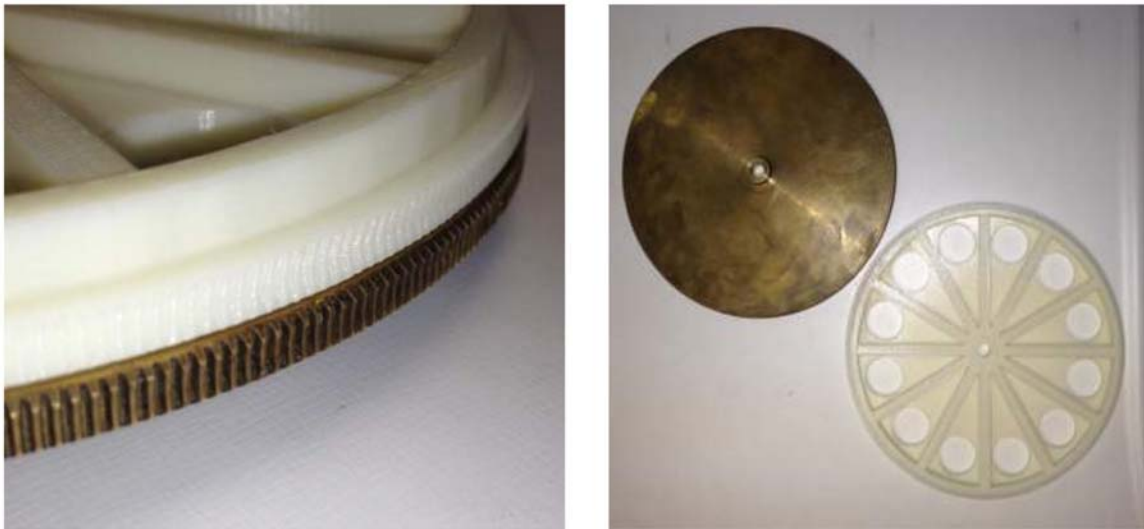
Figure 7.3D-Printed Replica Next to the Original Part TE-779 Test Fixture Used for Testing H-53 Stick Position Sensors Source: Lukesh, personal communication (2016).
